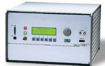
The Combination Wave Generator PG 12-805 is a combined impulse-current-/impulse-voltage generator which, for high-impedance loads,  $RL > 100\Omega$ , delivers a standard impulse voltage with waveform 1.2/50µs and, for short-circuited output, a standard impulse current with waveform 8/20µs.
